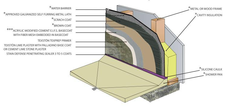
\*\*D.A.F.S.-Direct Applied Finish Systems Over Cement Board or Approved Backerboard
