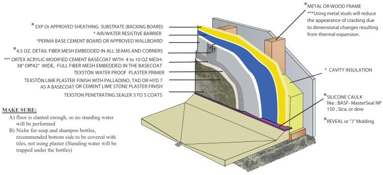
\*Supply by others \*\*This detail is for general information and guidance only. Final products detail is the responsibility of the project's designer/Architect. \*\*\* In order to add strength and flexibility as well as to tremendously reduce the appearance of cracks in the finish coat USE heavier mesh, like 10 oz. Instead of 4.5 oz. and use metal studs instead of wood
