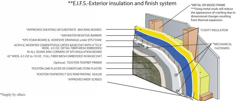
In order to add strength and flexibility as well as to tremendously reduce the appearance of cracks in the finish coat USE heavier mesh, like 10 oz. Instead of 4.5 oz..
