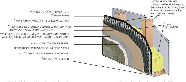
\*\*This detail is for general information and guidance only. Final products detail is the responsibility of the project's designer/Architect. \*\*\*Optional: In order to add strength and flexibility as well as to tremendously reduce the appearance of cracks in the finish coat USE heavier mesh, like 10 oz. Instead of 4.5 oz.
