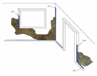
in between wall and object: Place and secure tape in a straight line over the objects away from the wall that going to be plastered. The gap needs to be as thick as the final finish thickness. For example:
